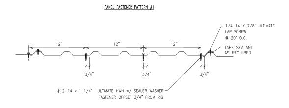
Figure 2. Low Rib X Metal Roofing Panel Secured to 16-Gauge Steel Purlins
