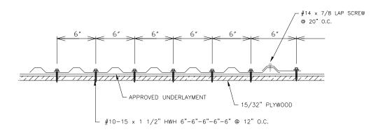
Figure 1. Low Rib X Metal Roofing Panel Secured to a 15/32" Plywood Deck
